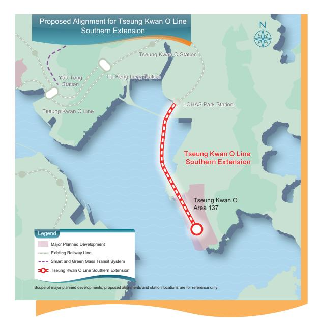
**2.4.10** The TKO Line Southern Extension, spanning approximately 4 km, aims to support the development of TKO Area 137 and provide a convenient and efficient mass transit system to the 135 000 new population. The Government recommends using the heavy rail system of the existing TKO Line as the basis, and extending the railway from the at-grade LOHAS Park Station southward to the underground station at TKO Area 137 via tunnels through the seabed
