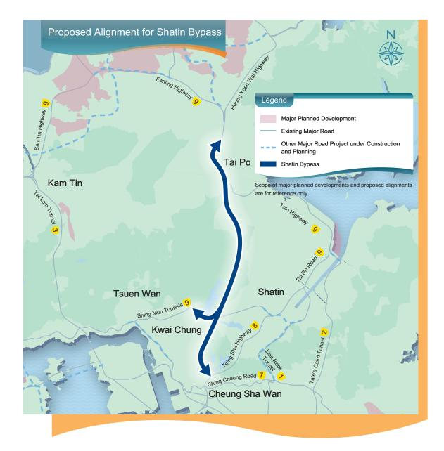
**2.4.18** The Shatin Bypass is approximately 15 km long. Compared with the existing Tolo Highway and the Tai Po Road, the Shatin Bypass will serve as a more direct north-south corridor, connecting the northeast New Territories with the urban areas of Kowloon. Its northern end will connect to the Fanling Highway in Tai Po, providing convenience not only for road users in the North District but also for residents in Tai Po, Tai Wo, Hong Lok Yuen, Lam Tsuen
