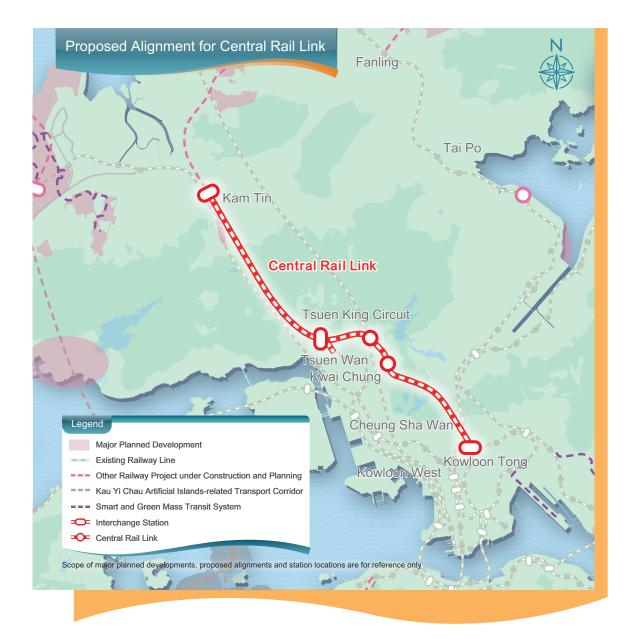
**2.4.5** The Central Rail Link (CRL) is an approximately 17-km railway connecting Kam Tin in Yuen Long and Kowloon Tong via Kwai Chung. It will link the Northern Metropolis and the Harbour Metropolis while supporting the sustainable development of the Northern Metropolis. Connecting to the existing and proposed railways, including the Tuen Ma Line, the Tsuen Wan Line, the Kwun Tong Line, the East Rail Line, the NOL, the NOL Eastern Extension
