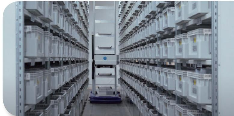
***24-hour-operated autonomous guided vehicles were purchased through the Pilot Scheme to save warehouse space and labour costs***
