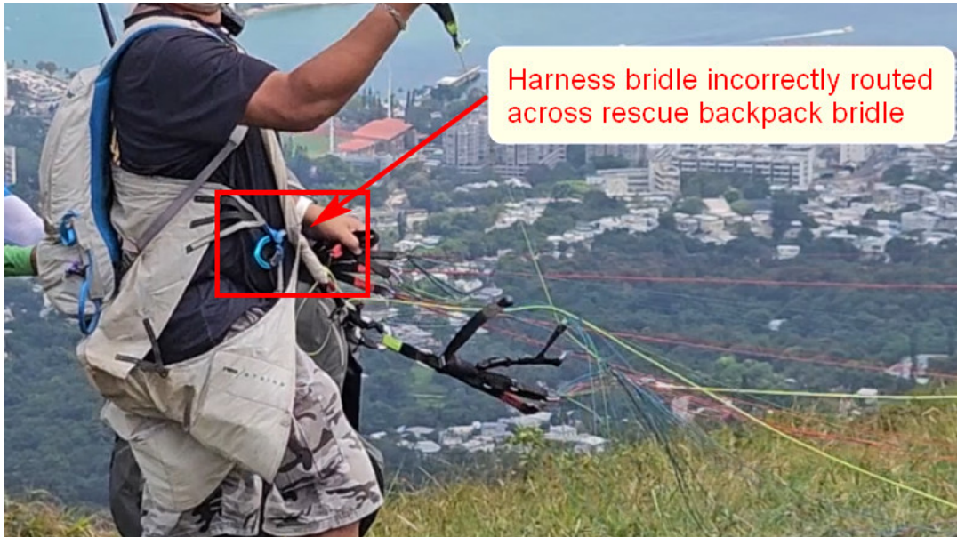
Figure 18: Bridle of Pilot's Harness Crossing That of the Rescue Backpack
