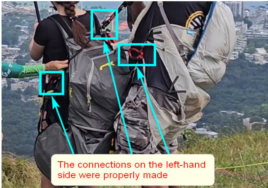
Figure 16: Spreader and Harnesses Connection on the Left-hand Side
