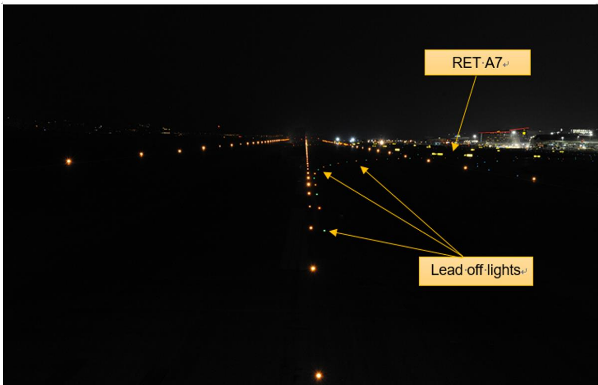
Photo 2: Lead off Lights Guiding Aircraft to RET A7
