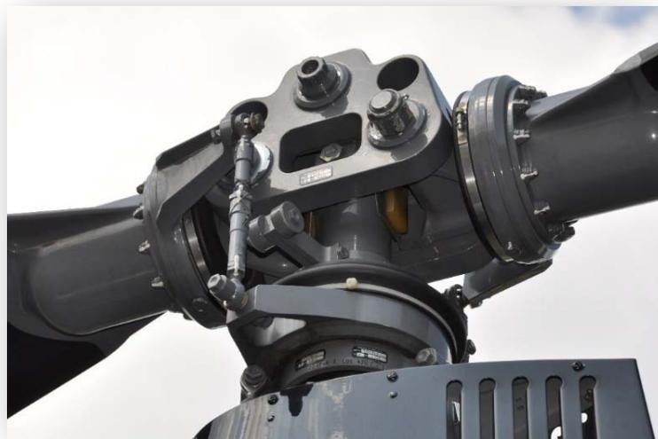
**Figure 16: R44 Main Rotor Head**
