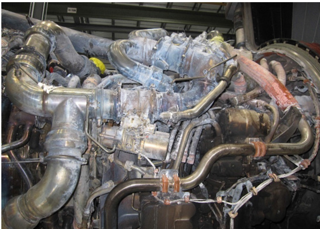
Figure 16: Right Side Close-Up of Thermal and Fire Damage
