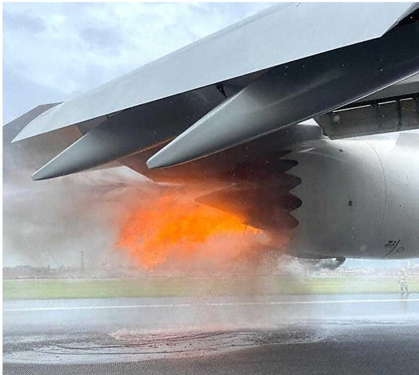
Figure 12: No.1 Engine Ground Fire
