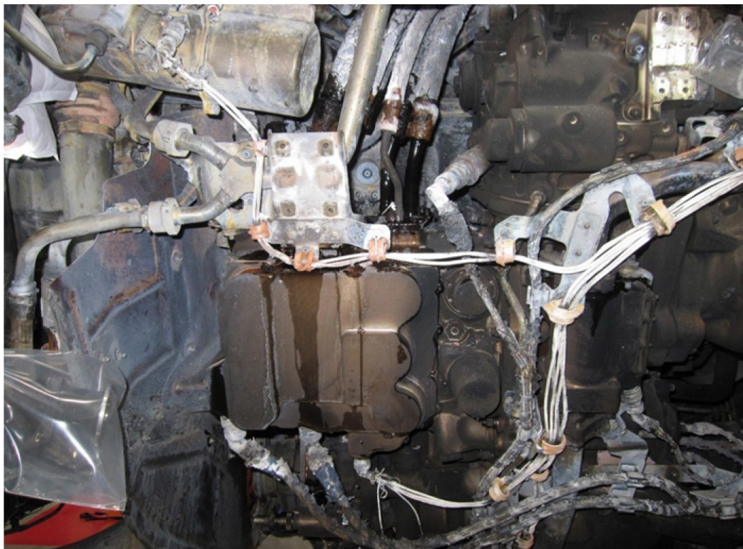
Figure 23: Fuel Leaking from Multiple Locations of FMU
