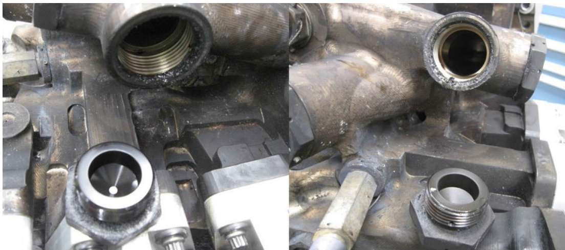
Figure 42: PB2 Bypass Packings Consumed
