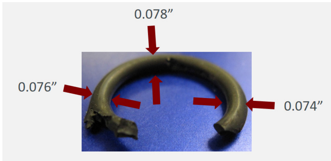
Figure 43: Damaged P1 Bypass Valve Port Fitting Packing
