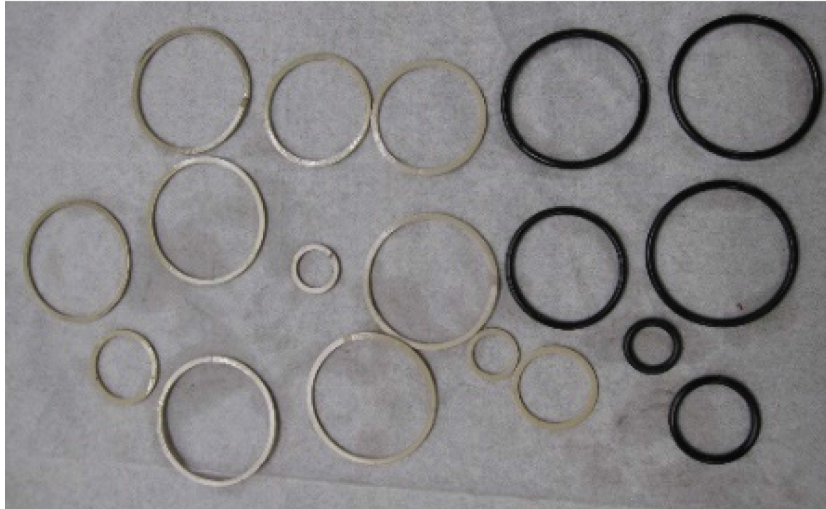
Figure 31: Condition of Packing & Back-up Split Rings
