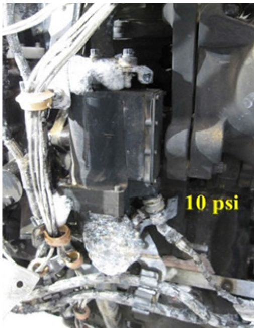
Figure 26: Leaking from Top and Bottom of FFT
