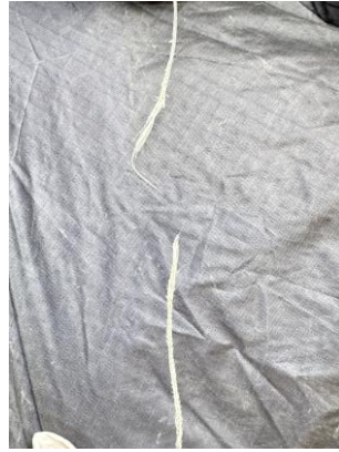
Figure 20: Right-hand C6 Line Broken
