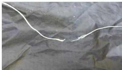
Figure 19: Left-hand StU Line Broken
